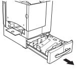
Make sure that the paper fits easily between the guides and the paper corners are under the left and right mediaseparating tabs and are not bent.
